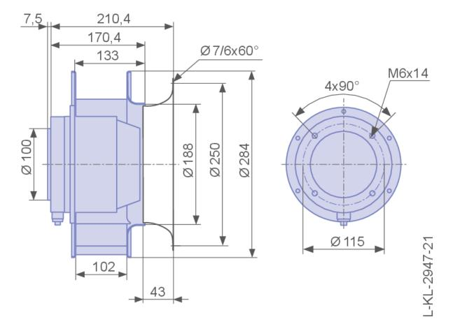
Dimensions in mm Shown drawing is just to show the dimensions of the fan.
